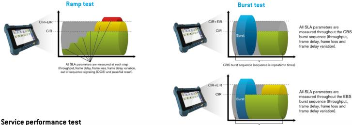
Once the configuration of each individual service is validated, the service performance test simultaneously validates the quality of all the services over time.
