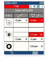
**Pass/Fail results in seconds:** With the press of a single button, FOCIS Flex auto-focuses, captures and centers the end-face image, applies Pass/Fail rules, displays image and Pass/Fail results. Captured Pass/Fai results are easily viewed in either Image or Table view.
