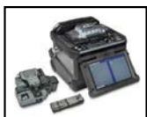
90R Fusion Splicer with CT50 Cleaver and RS03 Thermal Stripper
