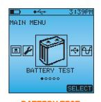
BATTERY TEST Standard, conductancebased battery testing.
