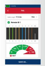
Cable test with remote attached shows remote ID number 1, length and pairing of each wire and cable performance of up to 2.5 Gb/s but failed the test due to a user-set limit of 10 Gb/s performance.
