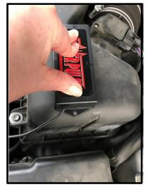
5) Mount the PowerPulse near the battery and not on the battery itself.
