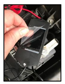
4) The circuit box can be mounted in various ways: with 2 rounded head screws, industrial adhesive or Velcro as shown above. (Attachment materials not included.)
