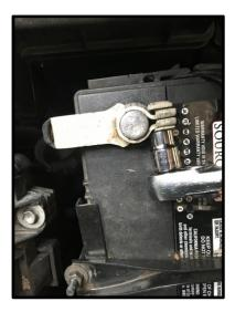
1) Unscrew the nut connected to the negative terminal.
