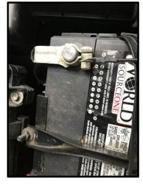
2) Slip the round metal lug at the end of the negative (black) wire onto the bolt and reinstall the nut tightly.
