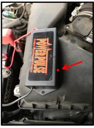
6) The flashing red LED indicates the Power Pulse is working.
