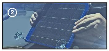
Make sure the suction cups are securely attached to the solar panel, and the bottom of the suction cups are clean. Mount the solar panel on the inside of the vehicle windshield where it will have direct access to sunlight.
