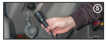
Push the OBD connector into the OBD port and ensure it's secure.
