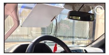
Let the solar panel cable hang down to the vehicle's OBD port.
