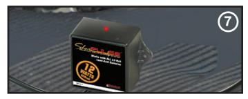
Make sure the circuit box's LED lights up indicating the solar panel is working at an optimum level. The LED dims when solar panel is in partial sunlight and you may need to move the solar panel into direct sunlight for maximum effectiveness.
