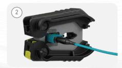
Insert the MTP® PRO Connector in the Polarity Change Port until audible "CLICK".
