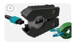
Compress the green Gripper handles <u>until they touch</u> and pull the Pin Exchanger out. Verify removal of pins.
