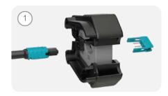
Insert unpinned MTP® PRO Connector in the Pin Change Port until audible "CLICK". <u>Do not compress the black handles during pin insertion.</u>
