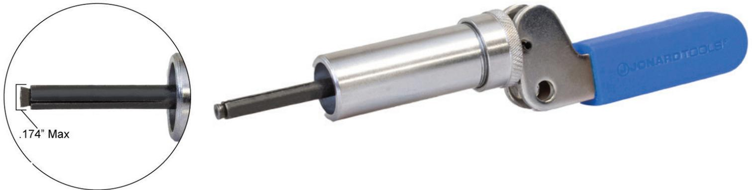
The Jonard Tools TTB-6 Barrel Lock Plunger Key is designed to unlock Channell LK03029817 and Highfield 93180775-S CATV barrel locks quickly and easily. It only works with these 2 types of locks with inside diameters from 0.176" to 0.196" (do not try to use for other purposes as it will not work). This barrel lock plunger features the following:
