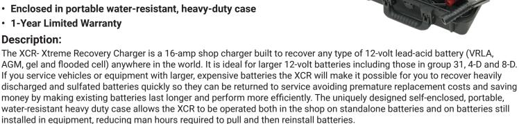
The Xtreme Recovery Charger uses PulseTech's patented Pulse Technology which emits a series of high frequency dc current pulses to reduce sulfation buildup which occurs over time as lead sulfates form on the battery plates during normal use. These sulfate deposits reduce the battery's ability to accept and keep a charge. Pulse Technology breaks down the deposits to improve battery performance and extend battery life up to three times.
