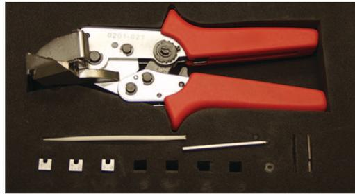
*The simplest and most reliable midspan access tool for loose buffer tubes.*
