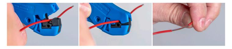
The Jonard Tools **BTR-6** Buffer Tube Ring tool provides quick access to fibers inside buffer tubes up to 6mm in diameter and will work with buffer tubes with wall thicknesses up to 1mm. The tool is light and durable with a hardened steel blade for long life. Includes hole for tethering.
