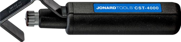
The **PATENTED** CST-1900 and CST-4000 Round Cable Strip & Ring Tools are designed for fast and precise removal of cable jackets from round cables. The CST-1900 removes cable jackets 3/16" to 1 1/8" (4.5 mm to 29 mm) in diameter and the CST-4000 removes cable jackets 3/4" to 1 5/8" (19 mm to 40 mm) in diameter. These round cable strippers feature the following:
