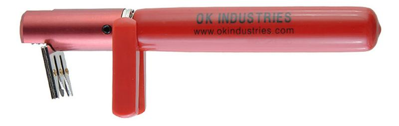
Designed to cut and strip off 7/16" to 1 1/8" length of wire, this cut-strip tool is the perfect tool for cutting and stripping 28-30 AWG (0.32-0.25 mm) wire for wire wrapping purposes. This cut-strip tool features the following:
