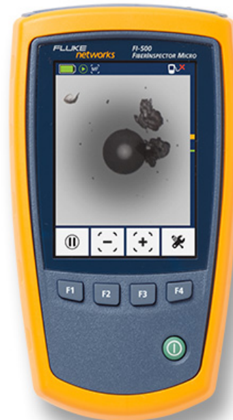
FI-500 displaying a dirty fiber endface
