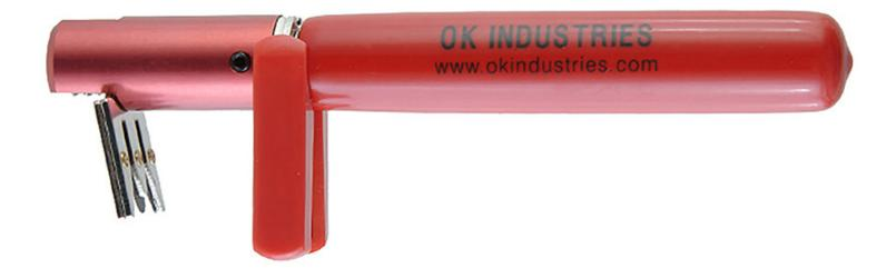
Designed to cut and strip off 5/16" to 9/16" length of wire, this cut-strip tool is the perfect tool for cutting and stripping 24-26 AWG (0.50-0.40mm) wire for wire wrapping purposes. This cut-strip tool features the following:
