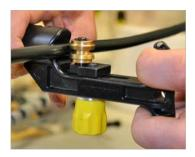
"T" handle design improves leverage & ergonomics during longitudinal or ring cuts.
