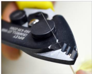
Precision made to prevent nicking or scratching the fiber.
