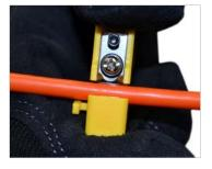
Reversible V-block provides optimal blade contact & stability during slitting operations.
