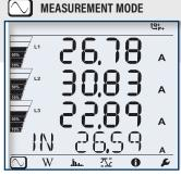
Hook up, voltage and current ratios and aggregation period can be configured from the front panel of the PEL 103.
