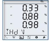
Total Harmonic Distortion (THD) can be displayed by phase or phase to phase. Neutral current THD can also be displayed.
