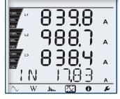
Max values for voltage, current (including neutral current), power and harmonics.
