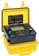
The Models 4620 and 4630 are built into a double case. This extra rugged construction provides double insulation, maximum field durability and ease of serviceability.
