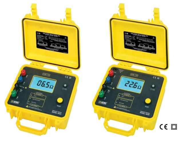
Digital Ground Resistance Tester Models 4620 and 4630 perform both ground resistance and soil resistivity tests. These testers measure from 0 to  $2000\Omega$ , and are auto- ranging, so they automatically seek out the optimum measurement range. Easy-to-use: simply connect the leads, press-tomeasure and read the results.
