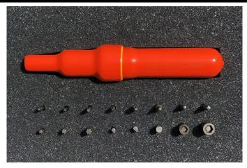
1050TSDK is a 1/4" hex adapter style insulated torque screwdriver kit from Cementex. It has a torque range of 10 to 50 ln. Lbs., works in the clockwise only direction. At only 8" long its' still small enough for limited space job tasks and the various tipped power bits keep the tips locked in place.
