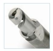
SCT tools core the dielectric and strip the aluminum sheath without scoring. The blade leaves a beveled outer conductor edge that eliminates O-ring damage, minimizing water migration.
