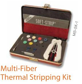
The MS-SK-1 kit contains the patented Soft-Strip® thermal stripper and components necessary for stripping the most popular ribbon types including 2-12 fiber encapsulated, bonded or ribbonized constructions. It is powered by an AC wall outlet adapter (order separately).
