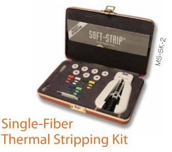
The **MS-SK-2** kit includes patented Soft-Strip® thermal stripper and components necessary for stripping discrete fibers with Cladding diameter up to  $140\mu m$  and Coating/Buffer diameter up to  $900\mu m$ . It is powered by an AC wall outlet adapter (order separately).
