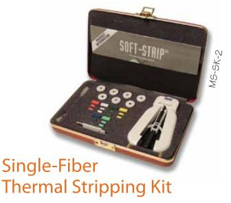
The **MS-SK-2** kit includes patented Soft-Strip® thermal stripper and components necessary for stripping discrete fibers with Cladding diameter up to  $140\mu m$  and Coating/Buffer diameter up to  $900\mu m$ . It is powered by an AC wall outlet adapter (order separately).
