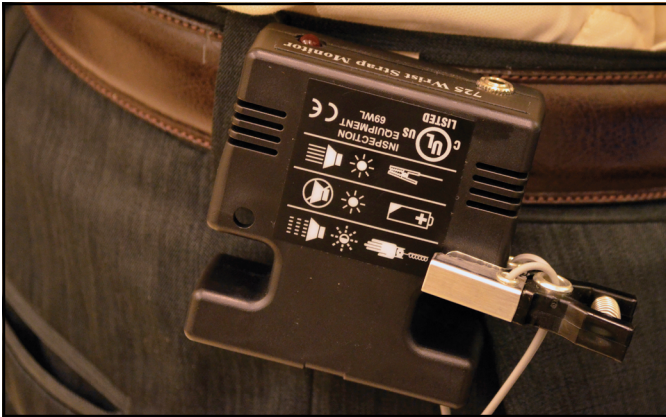
Figure 4. Using the 723 Belt Clip accessory
